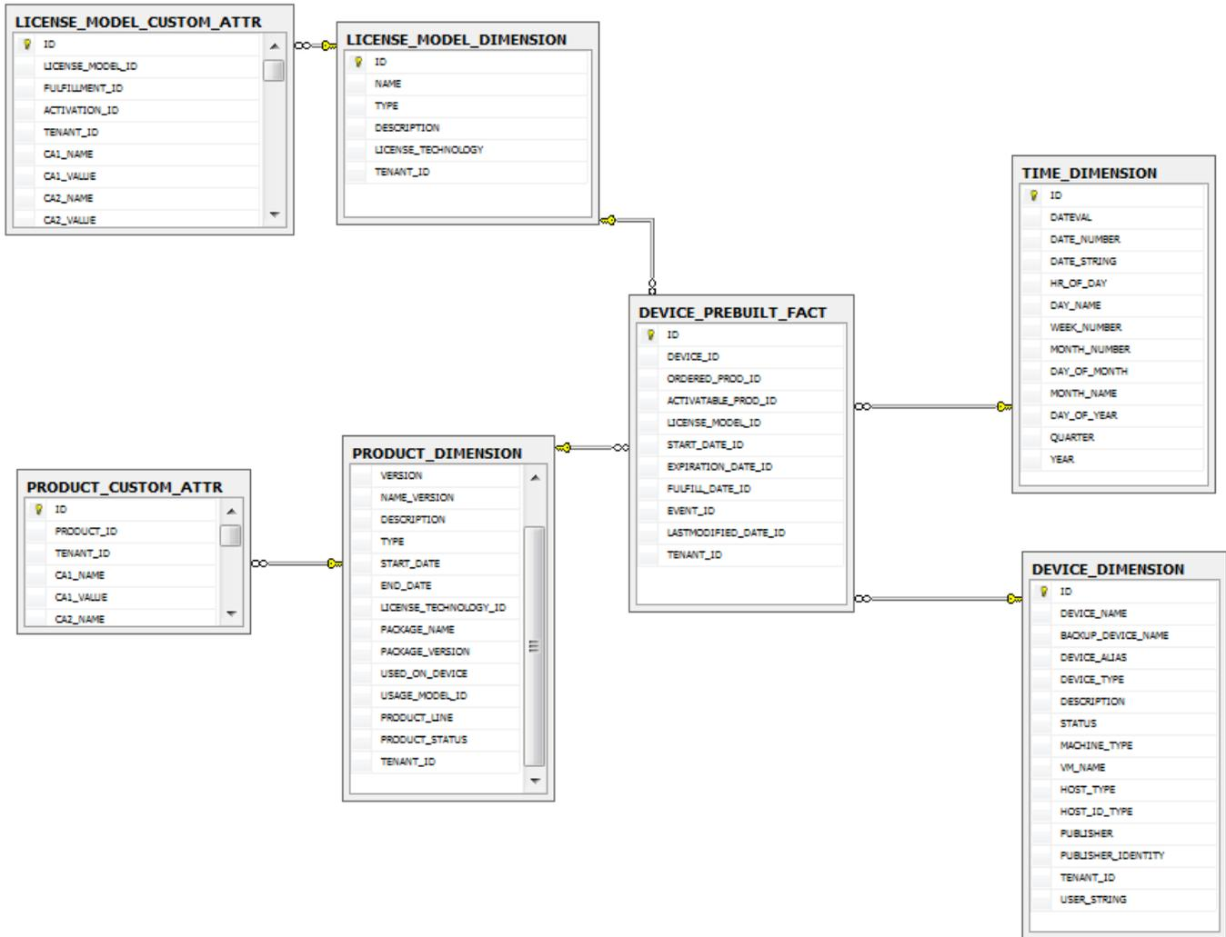
**Figure 3-5:** Entity Relationships for the DEVICE\_PREBUILT\_FACT Table
